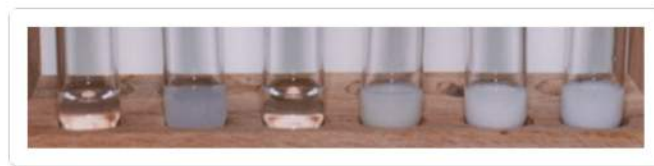
Figure 1: Test tubes containing several alkyl halides after the addition of NaI in acetone.
