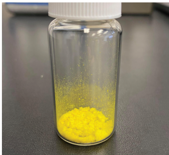
Figure 2. Isolated product, methyl 4-amino-3-nitrobenzoate ( 2 ), after wash and purification steps.
