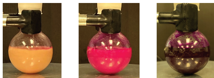
Figure 2. Left: suspension of 1 in THF immediately following addition of first drops of diethylamine. Middle: persistent pink/red color observed upon introduction of additional diethylamine. Right: final dark purple color caused by the formation of 2 .
