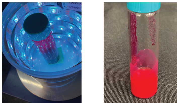
Figure 3. Left: solution of 2 in methanol with LED setup for cyclization reaction. Right: suspension of 3 in methanol with pink/red color caused by presence of minimal amounts of unreacted starting material.
