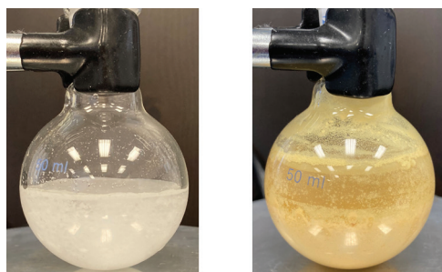
Figure 1. Left: suspension of furaldehyde in water prior to addition of 1,3-dimethylbarbituric acid. Right: precipitation of 1 as a bright yellow solid after addition of 1,3-dimethylbarbituric acid.
