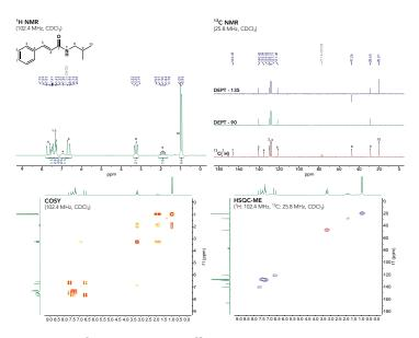
**Figure 2.** <sup>1</sup>H (102.4 MHz), <sup>13</sup>C (25.8 MHz), COSY (102.4 MHz) and HSQC-ME (<sup>1</sup>H: 102.4 MHz, <sup>13</sup>C: 25.8 MHz) NMR spectra of isobutylcinnamamide (3) in CDCl<sub>3</sub>. The asterisk in the <sup>1</sup>H spectrum represents the proton bound to the nitrogen in the amide.
