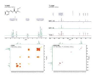
**Figure 3.** <sup>1</sup>H (102.4 MHz), <sup>13</sup>C (25.8 MHz), COSY (102.4 MHz) and HSQC-ME (<sup>1</sup>H: 102.4 MHz, <sup>13</sup>C: 25.8 MHz) NMR spectra of secbutylcinnamamide (**4**) in CDCl<sub>3</sub>. The asterisk in the <sup>1</sup>H spectrum represents the proton bound to the nitrogen in the amide.
