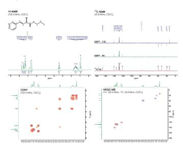
**Figure 1.** <sup>1</sup>H (102.4 MHz), <sup>13</sup>C{<sup>1</sup>H} (25.8 MHz), COSY (102.4 MHz) and HSQC-ME (<sup>1</sup>H: 102.4 MHz, <sup>13</sup>C: 25.8 MHz) NMR spectra of n-butylcinnamamide (2) in CDCl<sub>3</sub>. The asterisk in the <sup>1</sup>H spectrum 2 represents the proton bound to the nitrogen in the amide.
